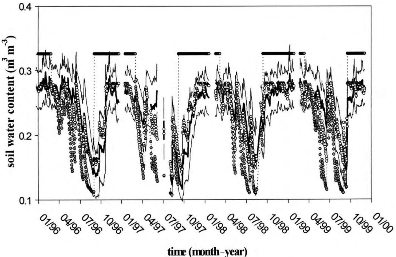
**Fig. 8. Influence of the position of the water table on the results of simulations performed with preferential flow at the 15-cm depth (Gray circles: water table set at the 3-m depth in winter and fall, and at the 100-m depth in summer and spring). For comparison purposes, results calculated by setting no influence of the water table are shown (open circles).**
