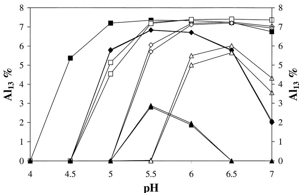
Fig. 7. Maximum and minimum contribution of  $\text{Al}_{13}$  to total dissolved Al in simulated surface waters as a function of pH, at  $T=0^\circ\text{C}$  (open symbols) and  $T=25^\circ\text{C}$  (dark symbols).  $\text{Al}_T = 10^{-3} \text{ mol l}^{-1}$  (squares),  $10^{-4} \text{ mol l}^{-1}$  (diamonds) and  $10^{-5} \text{ mol l}^{-1}$  (triangles).
