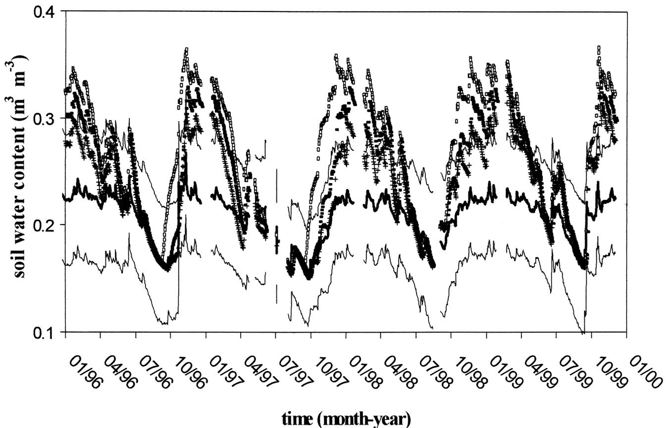
Fig. 5. Simulated water content at 60 cm using  $K_s$  and  $L = 0.5$  and by setting the water table during the wet periods (i.e., winter and fall) at the 2-m depth (open squares) and at the 3-m depth (filled squares). For comparison purposes, results calculated by neglecting the influence of the water table are given (cross). Mean and spread of the measured soil moisture content are shown (thick line: mean; thin lines: mean  $\pm$  sd).
