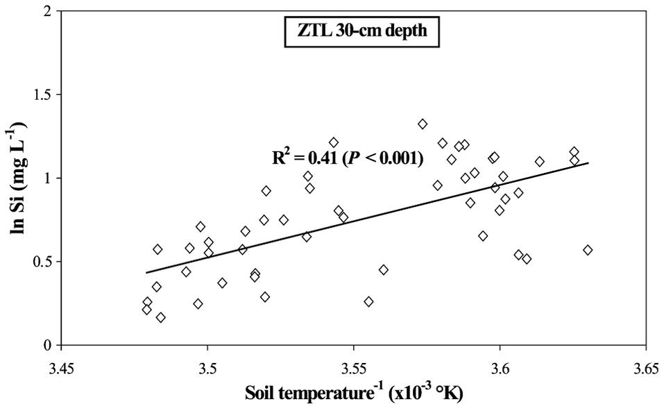
Fig. 6. Example of the linear relationship between the logarithm of silica concentration (lnSi) in leaching solutions and the inverse of soil temperature (1/T) expressed in Kelvin.
