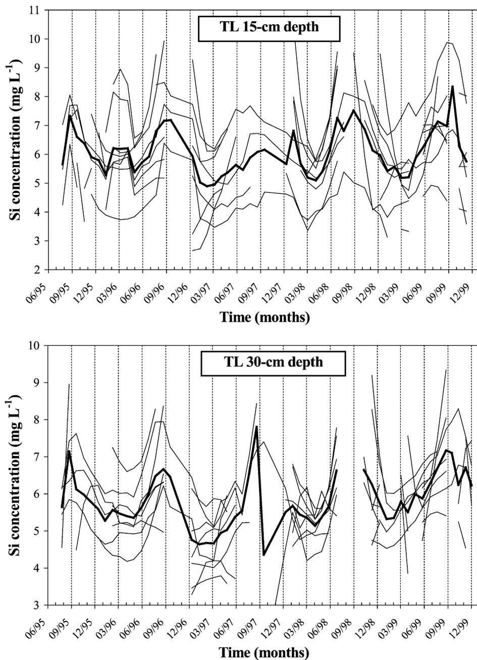
Fig. 2. Dissolved silica (Si) concentration according to time in capillary soil solutions collected by tension lysimeters (TL) at different soil depths (15, 30, 60, 120 cm).
