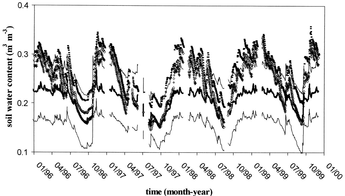
Fig. 6. Simulated water content at 60 cm using  $K_s$  and  $L = 0.5$  and by setting the water table at the 3-m depth, without readjusting the soil-dependent transpiration parameters (filled squares), after readjustment (open diamonds). For comparison purpose, results calculated by neglecting the influence of the water table are given (cross). Mean and spread of the measured soil moisture content are shown (thick line: mean; thin lines: mean  $\pm$  sd).
