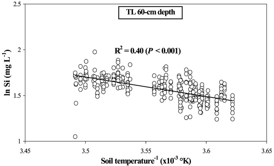
Fig. 5. Example of the linear relationship between the logarithm of silica concentration (lnSi) in capillary solutions and the inverse of soil temperature (1/T) expressed in Kelvin.
