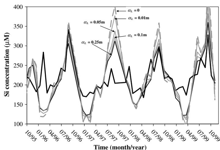
Fig. 6. Concentrations of Si as a function of time calculated with the model MIN3P for different values of the longitudinal dispersion coefficient, ranging from  $\alpha_L = 0$  (i.e. pure advection; dashed grey line) to  $\alpha_L = 0.25$  m (thin black line). Example given at 15 cm depth. Thick black line: measured concentrations.
