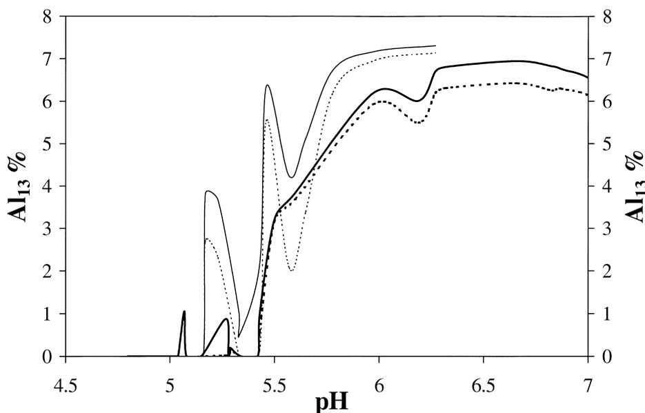
Fig. 1. Maximum and minimum calculated distribution of  $\text{Al}_{13}$  in soil solutions (15 cm depth = thick lines; 120 cm depth = narrow lines) as a function of pH, expressed in % of total dissolved Al. Calculations excluded the formation of HAS and organic complexes.
