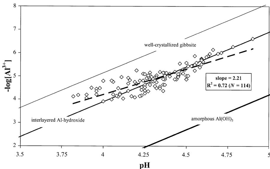
Fig. 6. Activity diagram for capillary solutions at the profile scale ( $T=25\text{ }^{\circ}\text{C}$ ) showing a significant linear relationship between the negative of the logarithm of the activity of  $\text{Al}^{3+}$ ,  $-\log[\text{Al}^{3+}]$ , and the  $\text{pH}$ .
