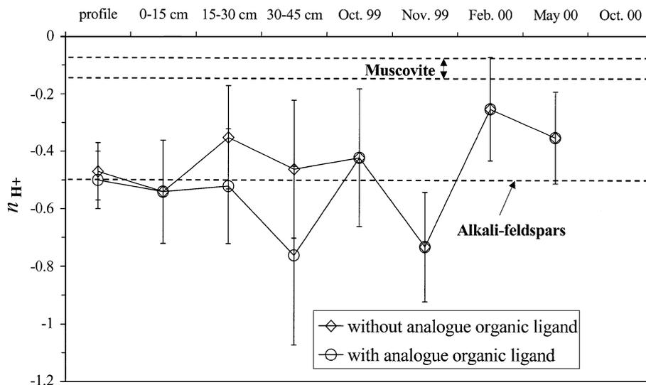
Fig. 7. Values of the linear regression parameter  $n_{H^+}$  (i.e. the slope of relationships between  $\log(\text{Si})$  and pH) calculated with different sets of data either considering the influence of organic ligands (open circles) or not (open diamonds). Error bars span a symmetric confidence interval of 95% of the mean value. Thick dashed lines represent the  $n_{H^+}$  values measured in the laboratory for primary minerals.
