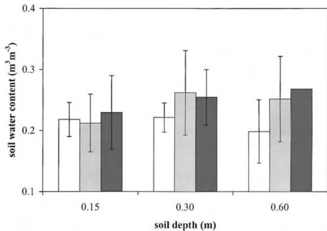
**Fig. 1.** Comparison of on-site control measurements of the soil water content at different soil depths. Error bars correspond to the standard deviation. White bars: mean value measured with the trase-system Soil Moisture time domain reflectometry (TDR) probes; light-gray colored bars: mean value measured with the Theta Probe Delta-T Devices; dark-gray colored bars: gravimetric measurements.
