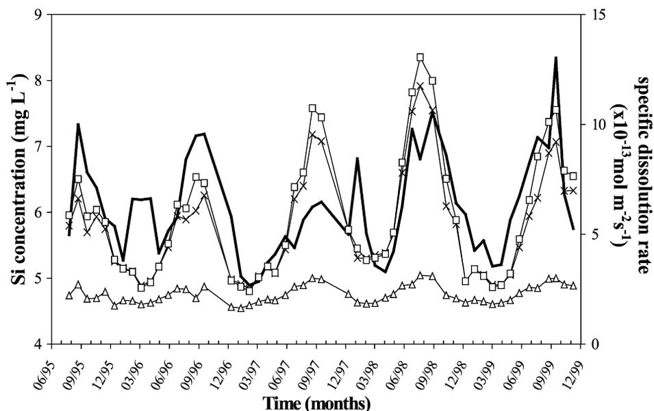
Fig. 13. Specific dissolution rates ( $r_d^*$ ) for K-feldspar (cross symbols), albite (square symbols) and white mica (triangle symbols) vs. silica (Si) concentration in capillary solutions. Example given at 15 cm depth.
