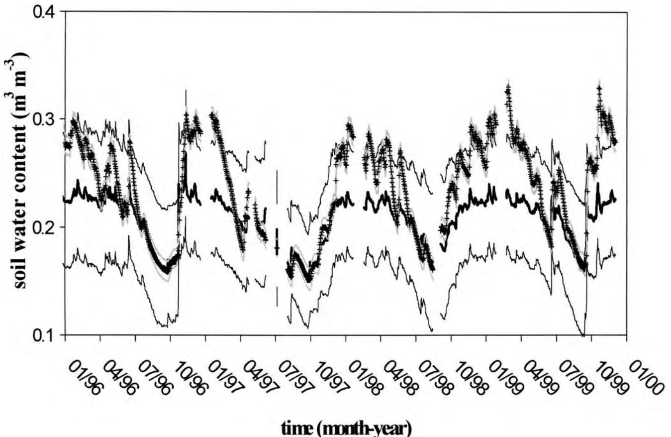
**Fig. 4.** Simulated water content at 60 cm by taking into account the prediction uncertainties given by ROSETTA (light curves) and using  $K_s$  and  $L = 0.5$ . Cross: simulation with the mean values of hydraulic parameters. Mean and spread of the measured soil moisture content are shown (thick line: mean; thin lines: mean  $\pm$  sd).
