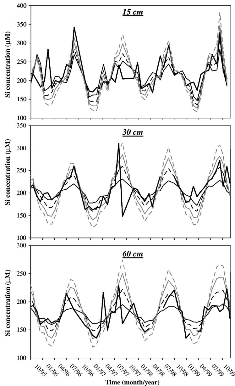
Fig. 7. Concentrations of Si as a function of time calculated with the model MIN3P by setting different values of the apparent activation energy ( $E_a$ ) of K-feldspar dissolution. Dashed grey line:  $E_a = 51.7 \text{ kJ mol}^{-1}$  (Blum and Stillings, 1995), continuous grey line:  $E_a$  25% decrease, thin dashed black line:  $E_a$  50% decrease, thin continuous black line:  $E_a$  75% decrease. Thick continuous black line: measured concentrations.
