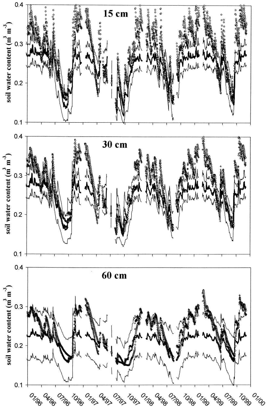
Fig. 3. Result of the simulations made with predicted hydraulic parameters and using the two types of prediction for hydraulic conductivity:  $K_0$  with  $L = 0.5$  (cross), and  $K_0$  with  $L \neq 0.5$  (circles). Mean and spread of the soil moisture content as measured by means of six time domain reflectometry probe replicates are shown (thick line: mean; thin lines: mean  $\pm$  sd).
