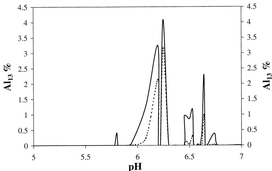
Fig. 3. Maximum and minimum calculated distribution of Al<sub>13</sub> in streamwaters as a function of pH, expressed in % of total dissolved. Calculations excluded the formation of HAS and organic complexes.
