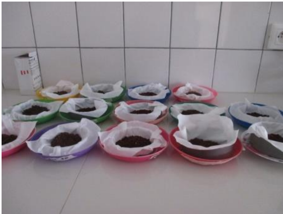
Photography 1.1: Active filtering of nematodes through fine cellulose wadding paper
