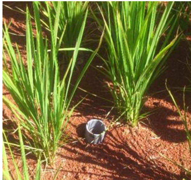
Photography 2.1: Intact soil core sampling
